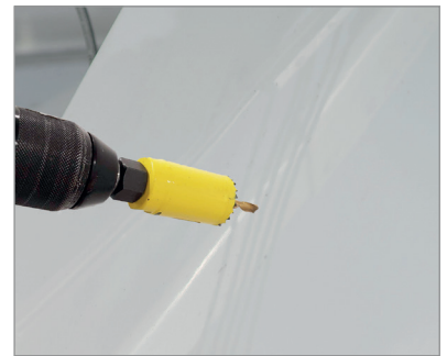
[Figure 13] Drill a 22 mm hole to the boat transom for the feedthrough of cables
