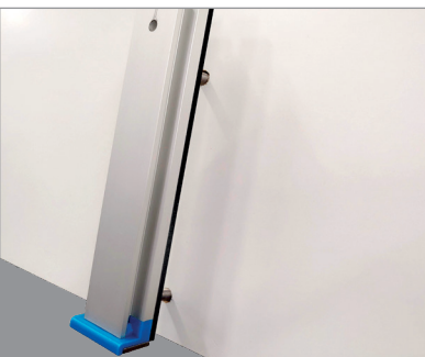
[Figure 9] Fit the bolts in the rail into the holes
